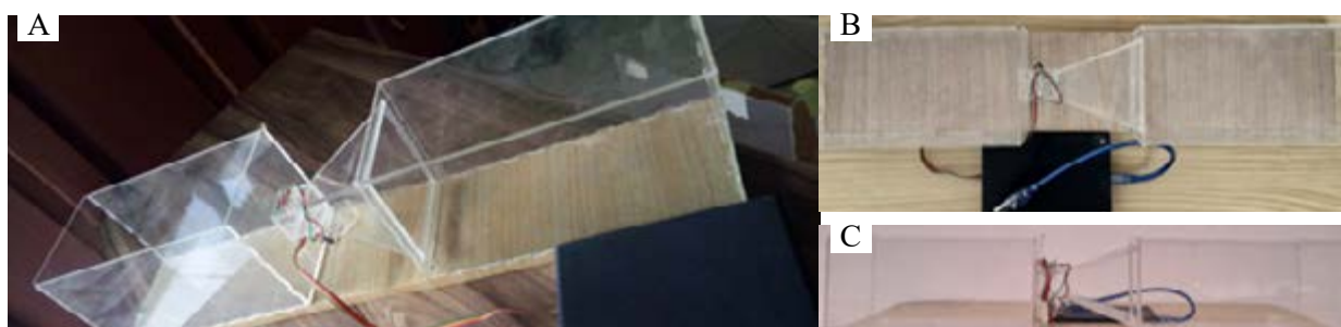
Figure 1. Experimental apparatus used to evaluate the accuracy of automatic insect counting sensors under laboratory conditions. The system consisted of two transparent acrylic chambers connected by a V-shaped tunnel equipped with an optical sensor. Adult fruit flies moved from chamber A toward chamber B containing a yeast attractant, allowing automatic counts to be compared with manual observations. A. Overall view; B. Top view; C. Side view.
